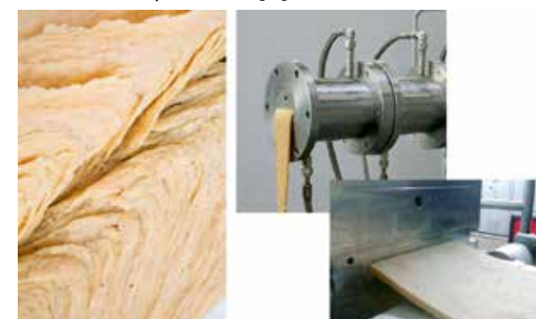
An image courtesy of CLEXTRAL showing fibrated plant based protein coming out of a twin screw extruder
